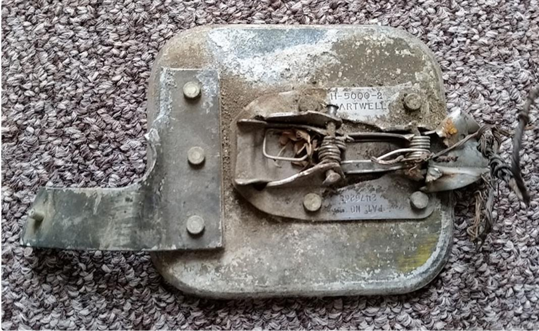
Part A: Latch Back. The Part number/patent number is for a **flush latch assembly**.
